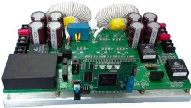
Fig. 9. Experimental prototype of the interleaved switched-capacitor bidirectional dc-dc converter.
